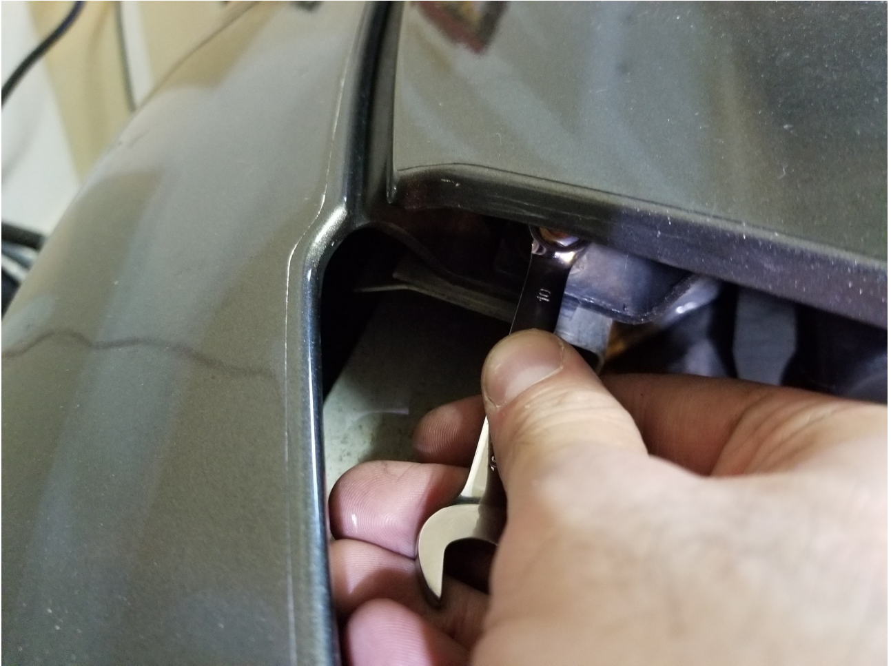
Figure 32: Slacken the nuts on either side that clamp the bumper in place
