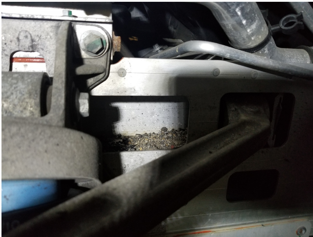
Figure 21: Inspect this crevice in the frame, behind where the top of the shock absorber is mounted. These were totally filled with pebbles on both sides of my car.
