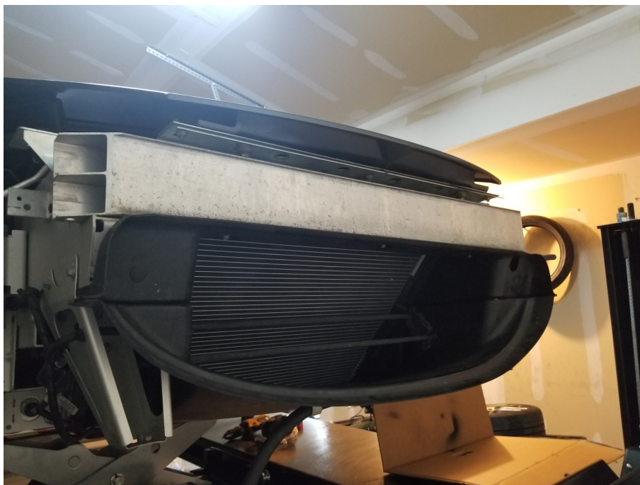
Figure 37: The plastic cowling that directs air over the condenser, radiator package, and PAS cooler pipes (if fitted)
