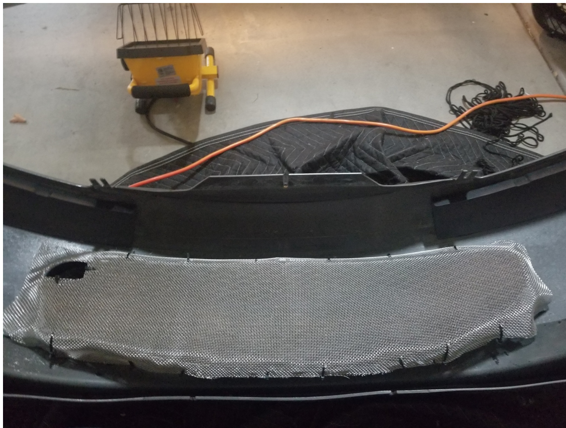
Figure 53: The partially installed mesh. Note the hole in the mesh, the zip-ties, and the unfinished left and right sides (needs more trimming, folding, and then zip-ties). If you leave the edges too long they can scrape the plastic, which should be avoided.
