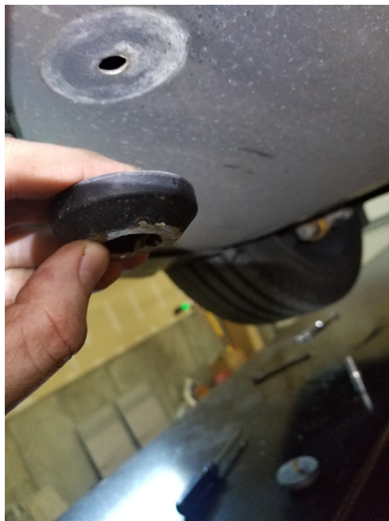
Figure 11: Each rubbing block is held on with 1x M6x16mm bolt (8Nm)
