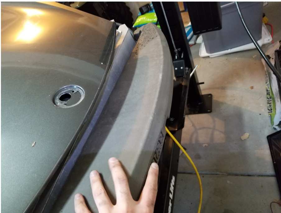
Figure 36: Remove this foam bumper pad
