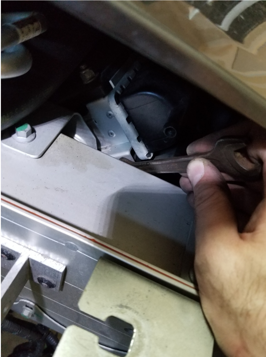
Figure 41: Remove the upper bolts to the condenser
