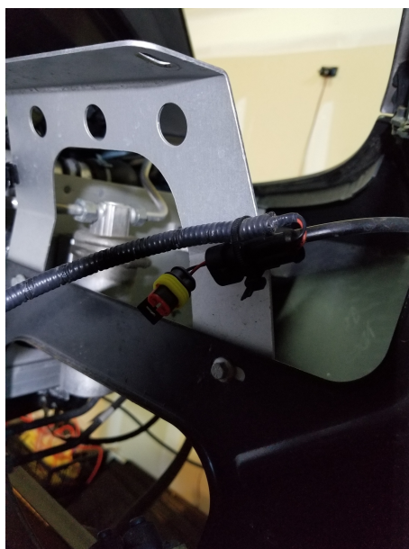
Figure 28: On either side of the car, clip the zip-tie that holds the wire harness that goes to the side lamp. Pictured is the LH side
