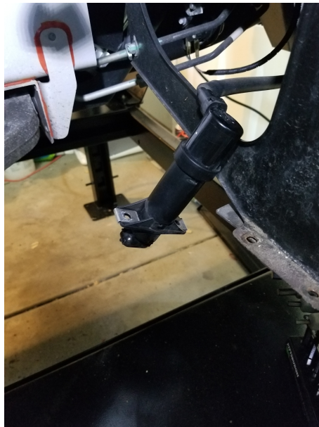
Figure 25: A dangling headlamp washer unit. It's much safer like this than trying to yank or pry a stubborn hose off the delicate hose fitting
