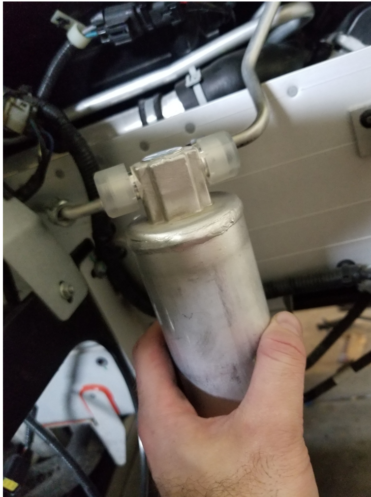
Figure 47: Install the new drier into the brackets, making sure that the flow arrow on the back is pointing in the same direction as the one you removed
