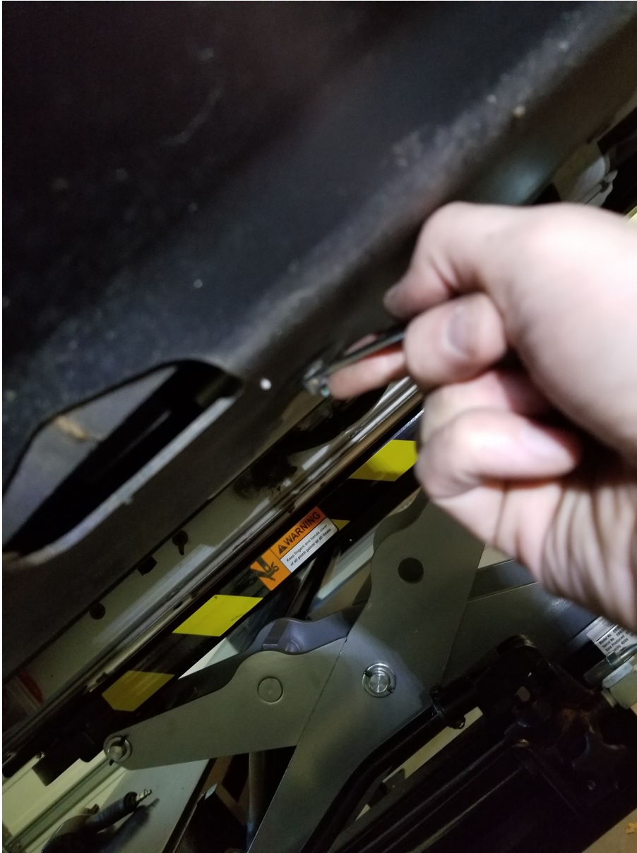
Figure 40: Remove two screws from the bottom of the cowling and three under the top lip
