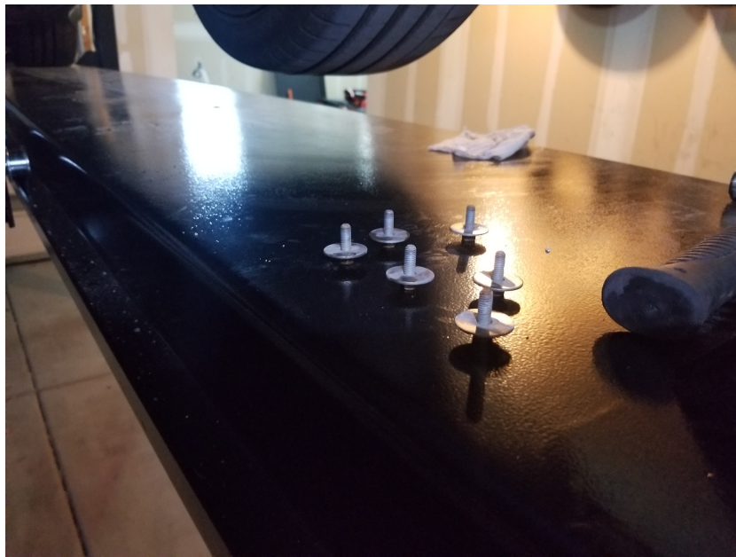
Figure 9: These are from the front bumper area, 8x M6x16mm (two not pictured), (8 Nm). Don't lose the captive nut clips that remain on the undertray
