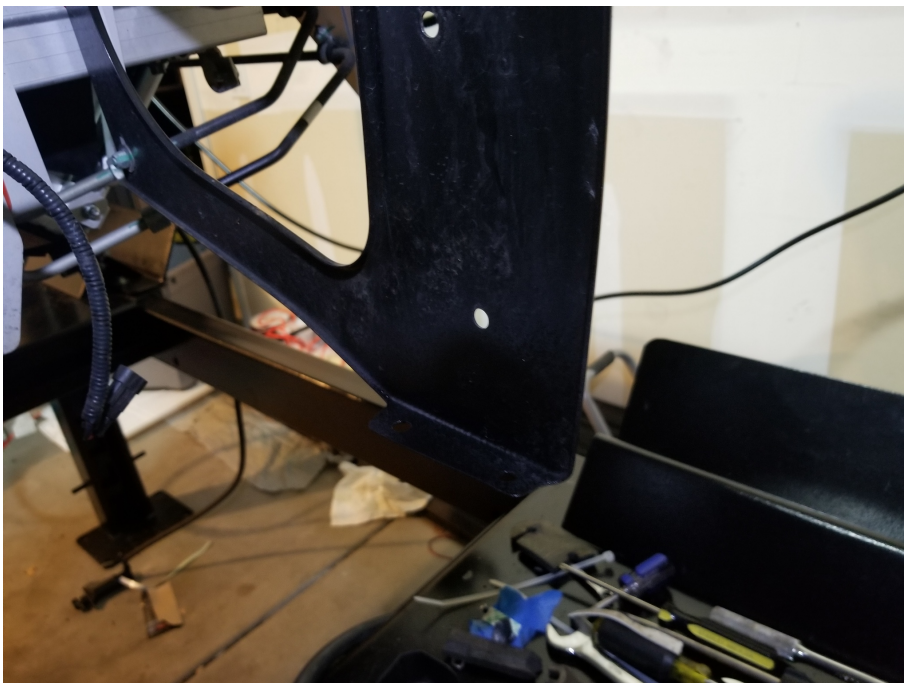
Figure 20: Support that's been treated with rust converter (and I think I sprayed some underbody coating on this one too). Note that the bumper has already been removed in this photo.
