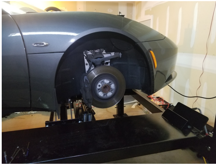
Figure 15: Removing the wheels is similarly straight-forward. Loosen them on the ground first
