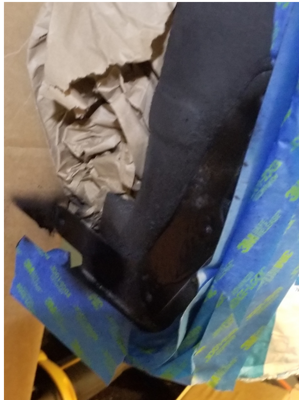
Figure 19: Masked mudflap bracket with rust converter applied
