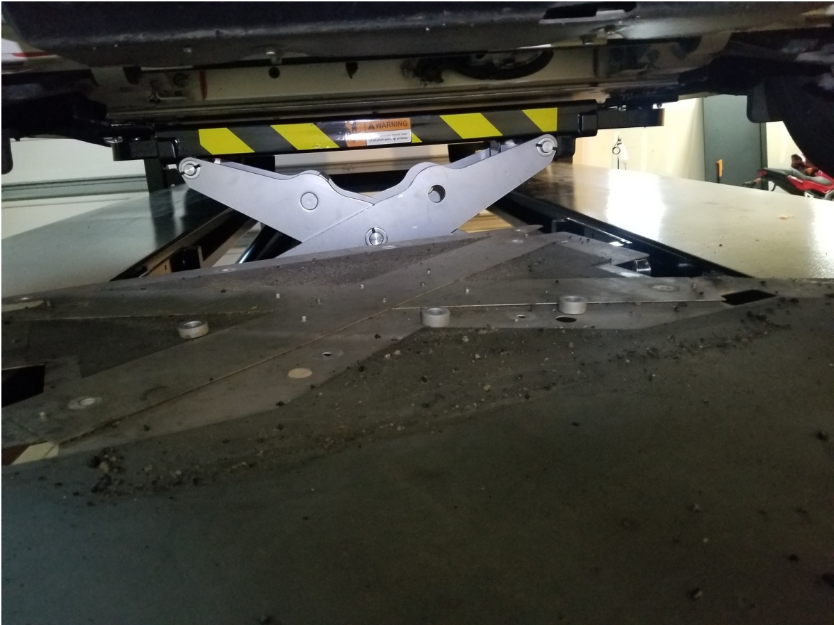
Figure 12: Slide the undertray towards the back of the car and wiggle the front out from under the bumper, being careful not to bend or crack the bumper. Here's the removed undertray filled with road grit. You can see some of the various spacers. These fit on in specific locations later
