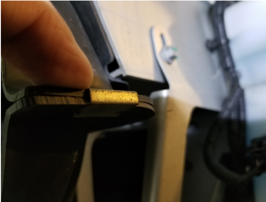
Figure 38: Using a screwdriver and hammer, poke or slide these clips out from the cowling. There are four on each side.
