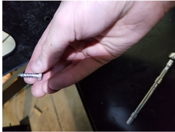
Figure 26: One of the two hex-head screws that hold the headlamp washer unit.
