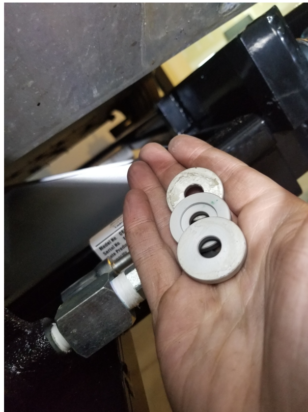
Figure 55: Close-up of spacers. There are four sizes that are placed in back-to-front: 4x 4.6mm, 2x 3mm, 2x 10.6mm, and 2x 13.7mm which are on the inner-most and most-forward area. Refer to service notes A. p.10
