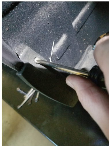
Figure 16: I found it easy to strip the screws for the mudflaps. You can replace them with M5x16 screws.
