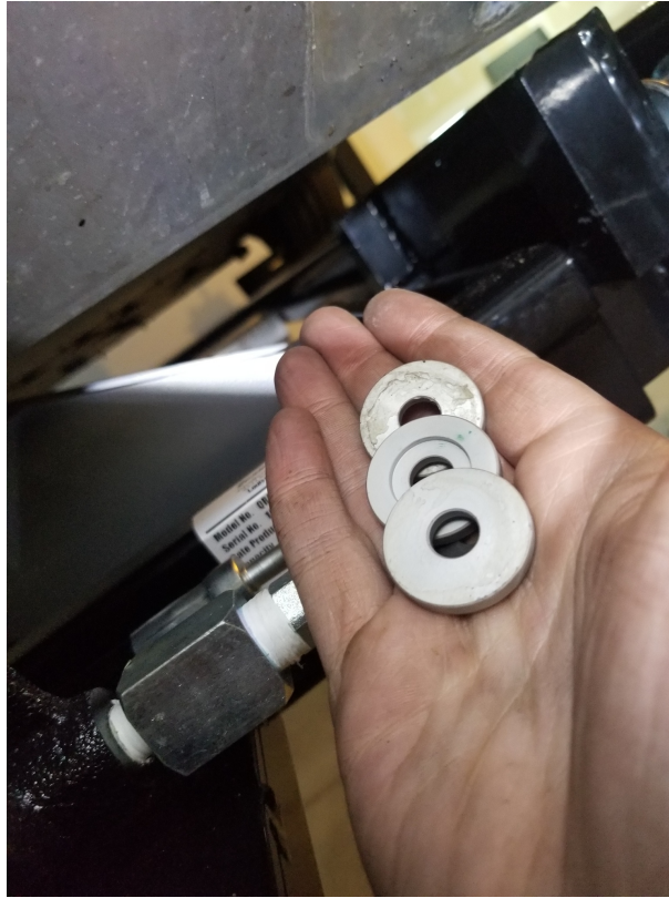
Figure 13: Close-up of spacers. There are four sizes that are placed in back-to-front: 4x 4.6mm, 2x 3mm, 2x 10.6mm, and 2x 13.7mm which are on the inner-most and most-forward area. Refer to service notes A. p.10
