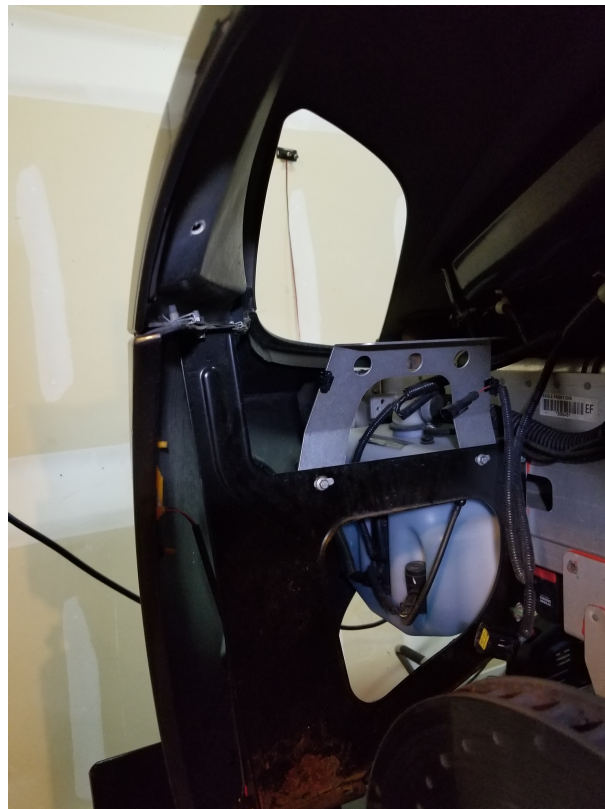
Figure 27: The area where the headlamp sits. You can see rust on the bottom of the support, and note the four bolts on the left side of the seam between the clamshell and the bumper, which will need to be removed in the next section.
