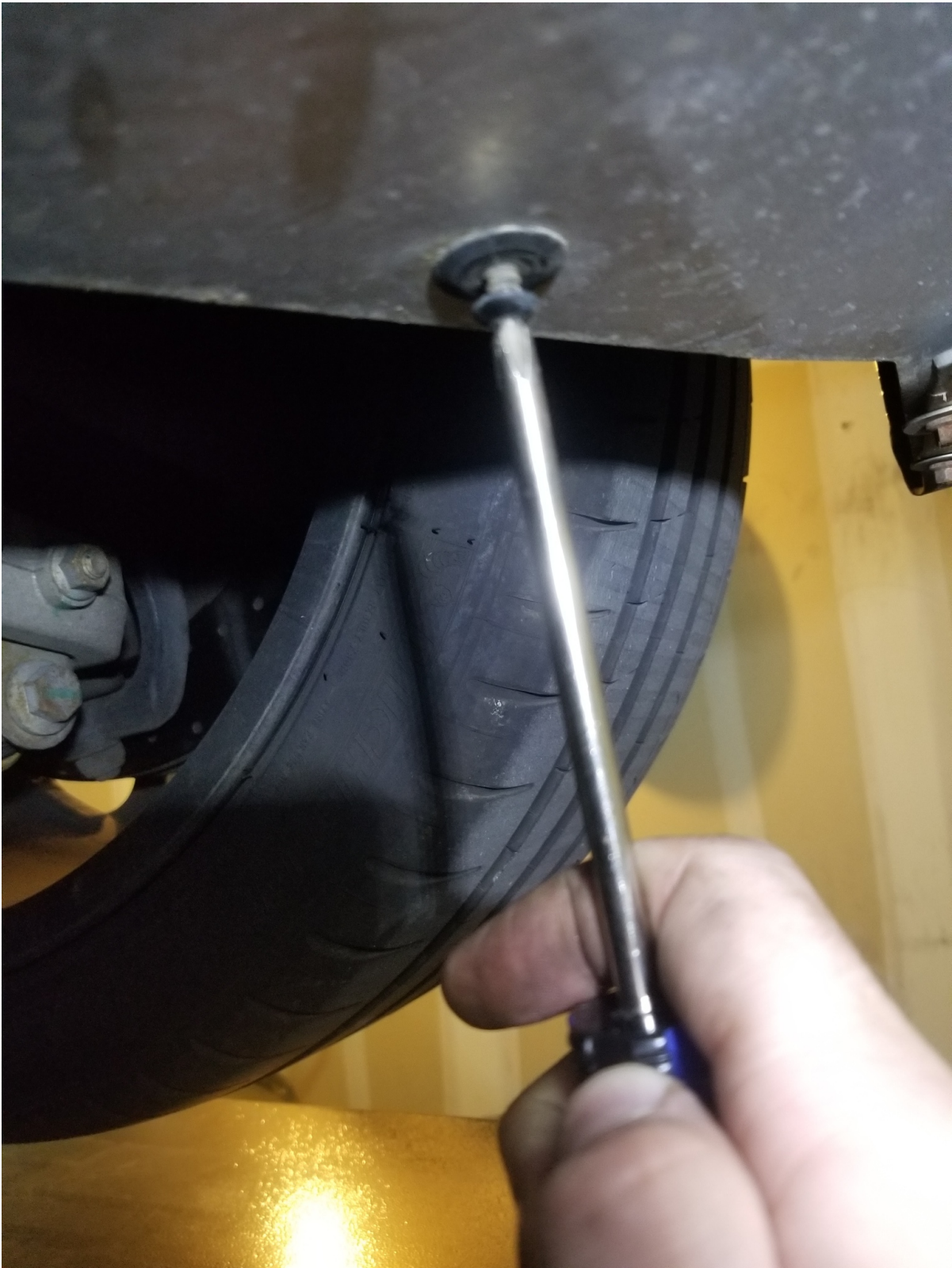
Figure 7: Each side has a push-fit rivet that goes to the wheel-arch liners
