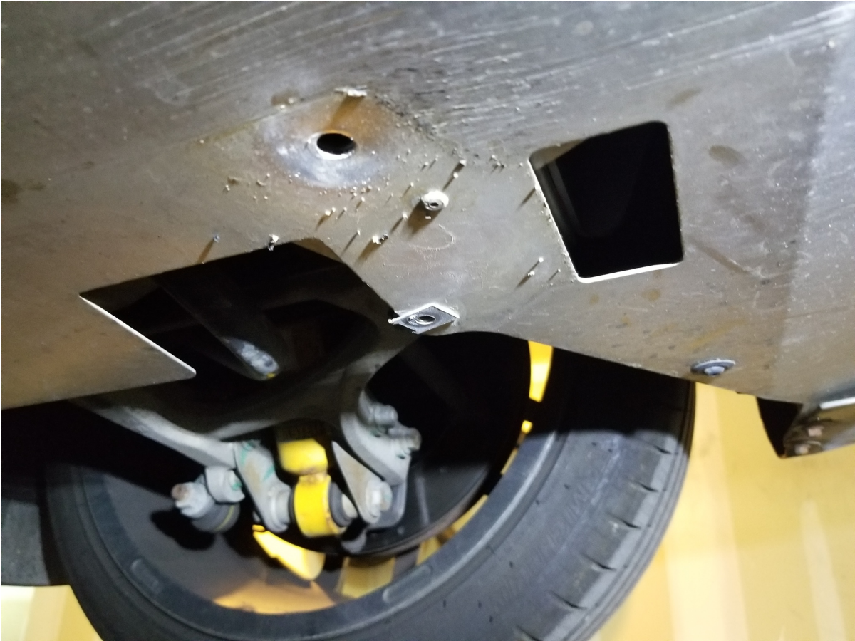
Figure 6: These side panels are held on with 2x M8x20mm bolts (12Nm) and 1x M8x30mm (12nM)
