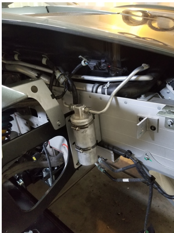
Figure 51: The new drier and condenser with the lines reattached
