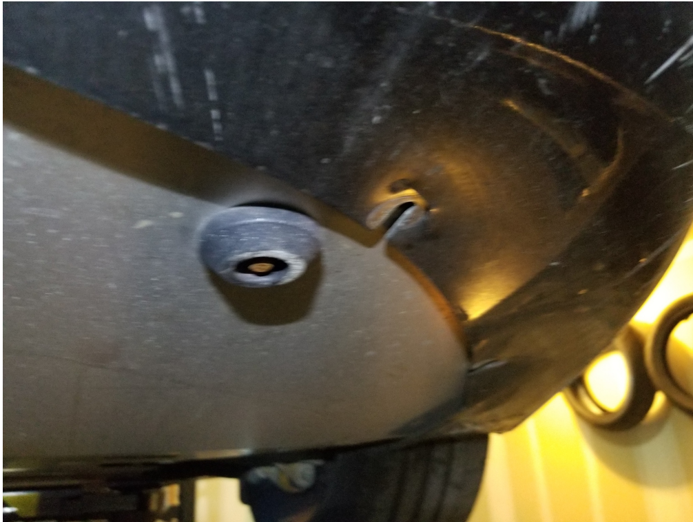
Figure 10: Front bumper M6x16mm bolts removed, and you can see the undertray rubbing block. You can also notice a crack in the bumper's plastic, perhaps the result of flexion while bottoming out
