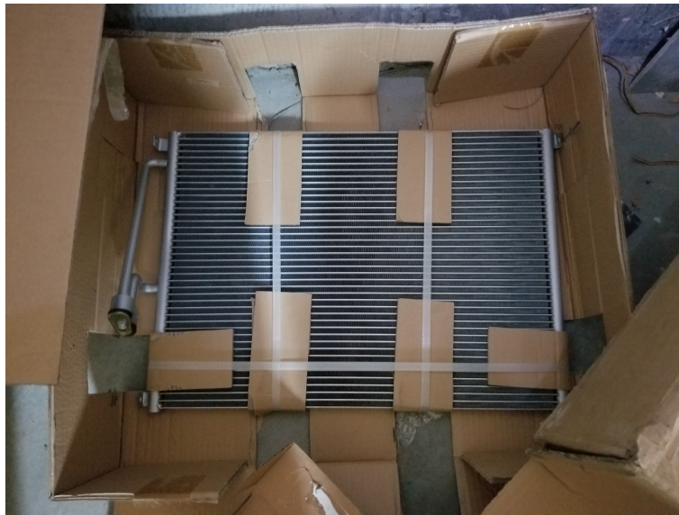
Figure 48: New condenser! Note the plate that keeps the pipes sealed—become familiar with how to loosen it, and you can slacken the bolt/screw now, to make it easier in a few moments. Also take care to not damage the heat-exchanging fins.
