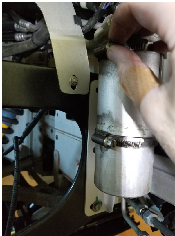
Figure 46: You can also unscrew the clamps that hold the drier to the bracket and remove it now. Note the flow arrow on the back of the drier! I don't have a photo to prove which direction it should go in, sadly, and I don't want to guess at this point.
