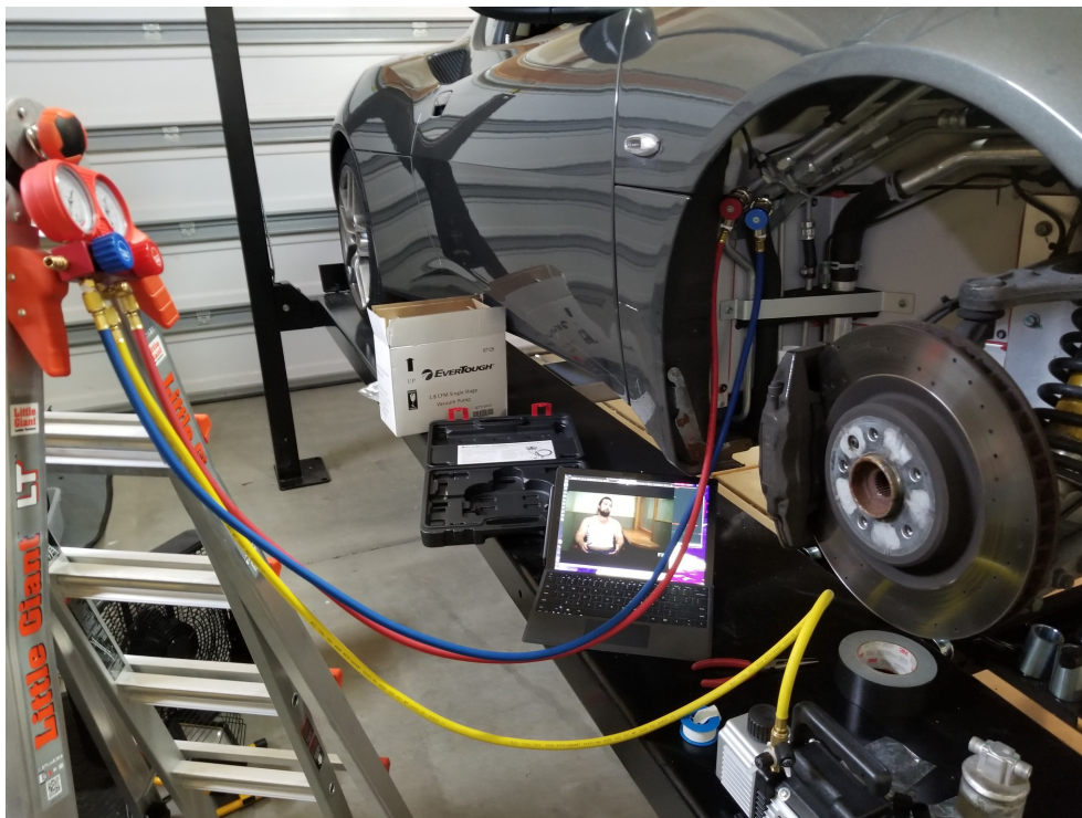
Figure 52: The manifold set attached to my car. I watched about five seasons of It's Always Sunny in Philadelphia while doing this job. The uncapped drier in the bottom right of the picture is the old drier. Never expose the AC components to air for any longer than you have to! Especially the drier, which contains a silica desiccant that will rapidly become saturated if exposed to atmosphere.
