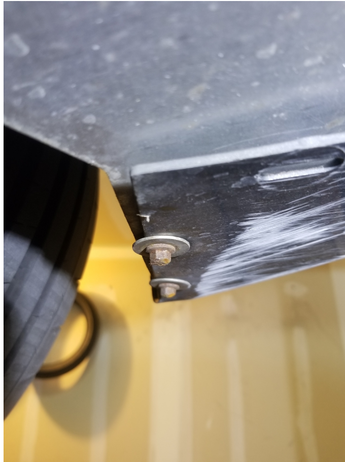
Figure 8: Each side has 2x M6x16 screws, washers, and flange nuts. Mine required PB blaster and were scraped up from bottoming out the car. You may need to remove these after removing the wheel arch liners
