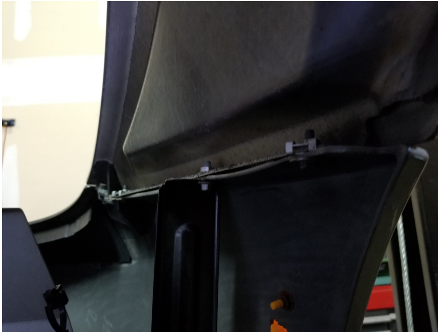
Figure 30: Remove four bolts from each side of the bumper. The central one is an M6x16 screw & nut and goes through the aluminum support. The other three are M5x16 screws & washers that go into clips
