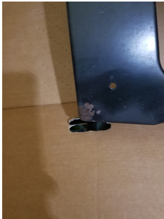
Figure 18: Inspect the bottom of the supports near the wheel arch. Mine had rust under the paint. Either before or after removing the bumper, scrape the affected paint and rust away with a wire brush, clean the dirt, and spray with rust converter. Be sure to mask the surrounding area.
