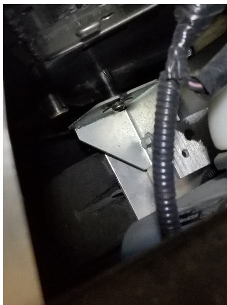
Figure 23: Detach the headlamp wire connector by squeezing down on the top retainer and pulling back with light force.
