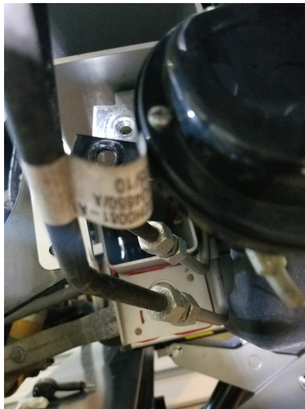
Figure 39: Remove the horns from either side of the cowling. Pictured here is the bracket that holds them in place; I removed the screw from the bracket, withdrew the horns, then reattached them to the bracket for safe keeping.
