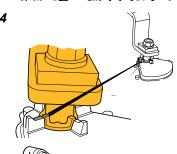
5. Push the fixed end joint of the shift rod onto the ball of the shift actuators lever arm ball mounting
