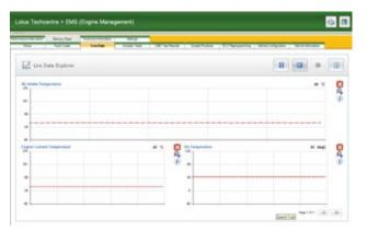
Once you are certain that the sandwich plate thermostat has opened allowing the transmission fluid to circulate completely around the external cooling system have then allowed the fluid temperature to drop to 40°C you can then check the fluid level as described on the next page.
