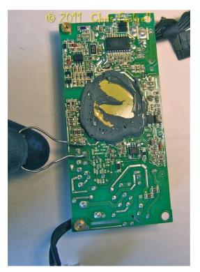
The two bulging capacitors are the ones mentioned at the start. Bulging capacitors are usually dead ones. We will remove these using skill, tenacity and a decent sized soldering iron, along with other implements of circuit board dismantlement.
