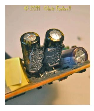
Cut the grey stuff away with your not-too-sharp knife. Waggle the two capacitors up and down (they can't touch you for it) and the solder, if any remains, will crack and break free.
