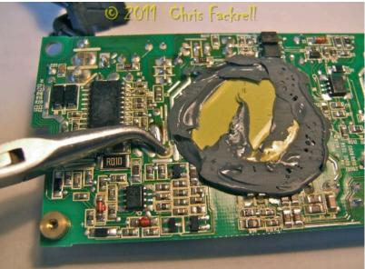
The soldered connections of the two capacitors are along here. The terminal nearest to the yellow centre component
