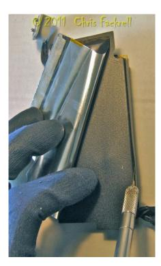
Take the trusty knife and again, gently slice the two parts, apart. The glue is vile here and will happily 'snag' the blade. Gently twisting the blade will help to pry them open.
