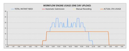
In the chart, the blue line shows the instant computing need if unlimited computing resources were available. The orange line shows CPU usage based on the number of Xgrid nodes available. In this case, there are three Xgrid nodes, each with four CPUs.
