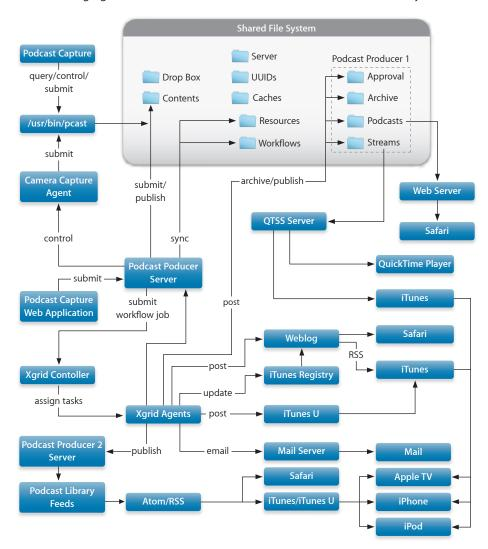
The Podcast Producer system consists of the following main components:
