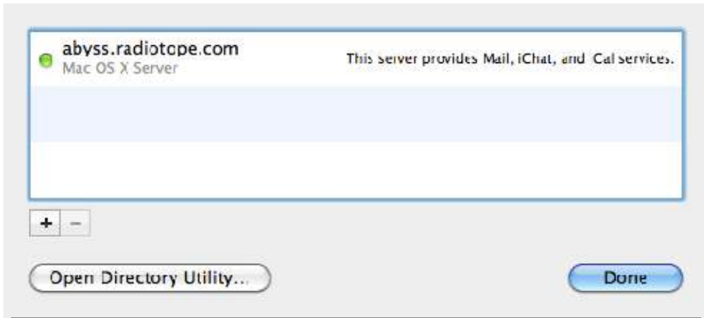
Figure 6-2. Directory Service sheet showing an active binding to an Open Directory server
