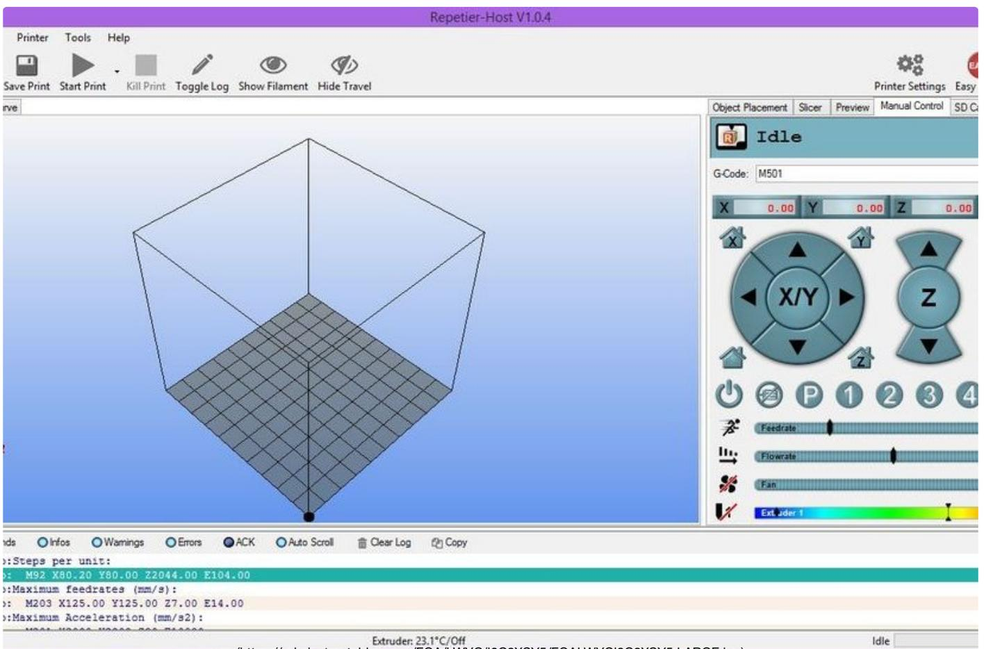
After opening Repetier and connecting your 3D printer, select the manual control tab. Next turn off easy mode and hit the toggle log button(if you're using the most recent version of Repetier), then type into the G-Code: “M501” then press enter or hit send (a bunch of information will be added to your log, at the bottom of the screen)
